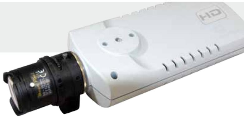
IndigoVision's cameras enable simple and easy deployment of IP based video systems as they only require a single CAT 5 cable for connection to the network. The built-in Power-over-Ethernet support allows the camera to be powered directly from the network, reducing installation costs.
